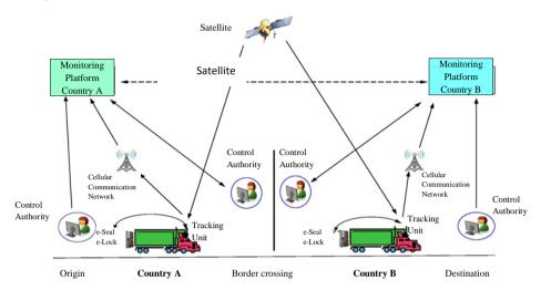
This model demonstrates that the integrated use of ICT can secure and facilitate trade and transport, while taking care of the concerns of control authorities. A vehicle-tracking system based on the model can give control authorities the confidence they need to open up more land routes for international trade and transport while also enabling transport operators to manage their operations efficiently.
